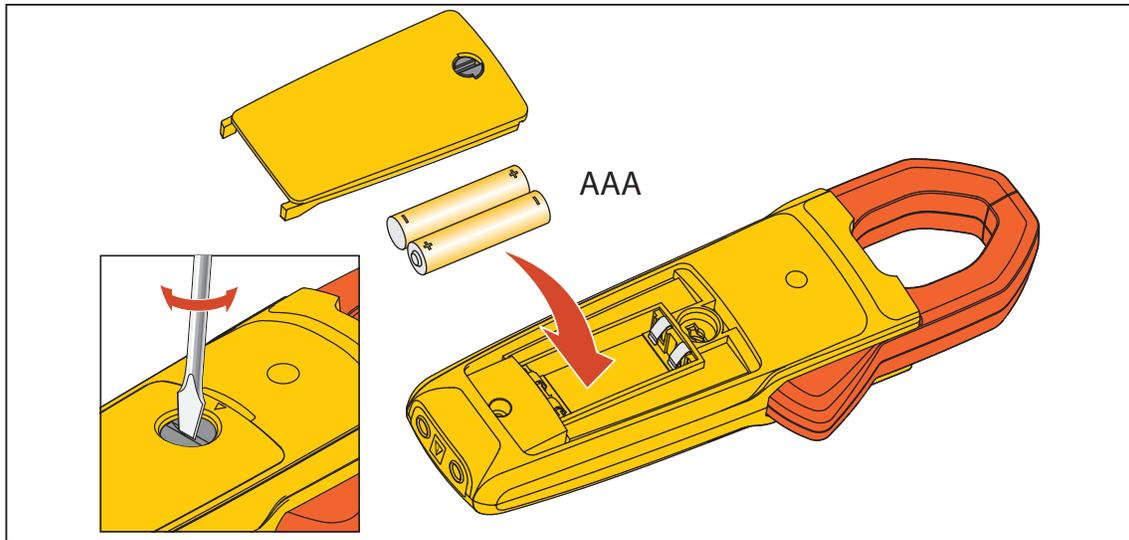
Figure 2. Battery Replacement
