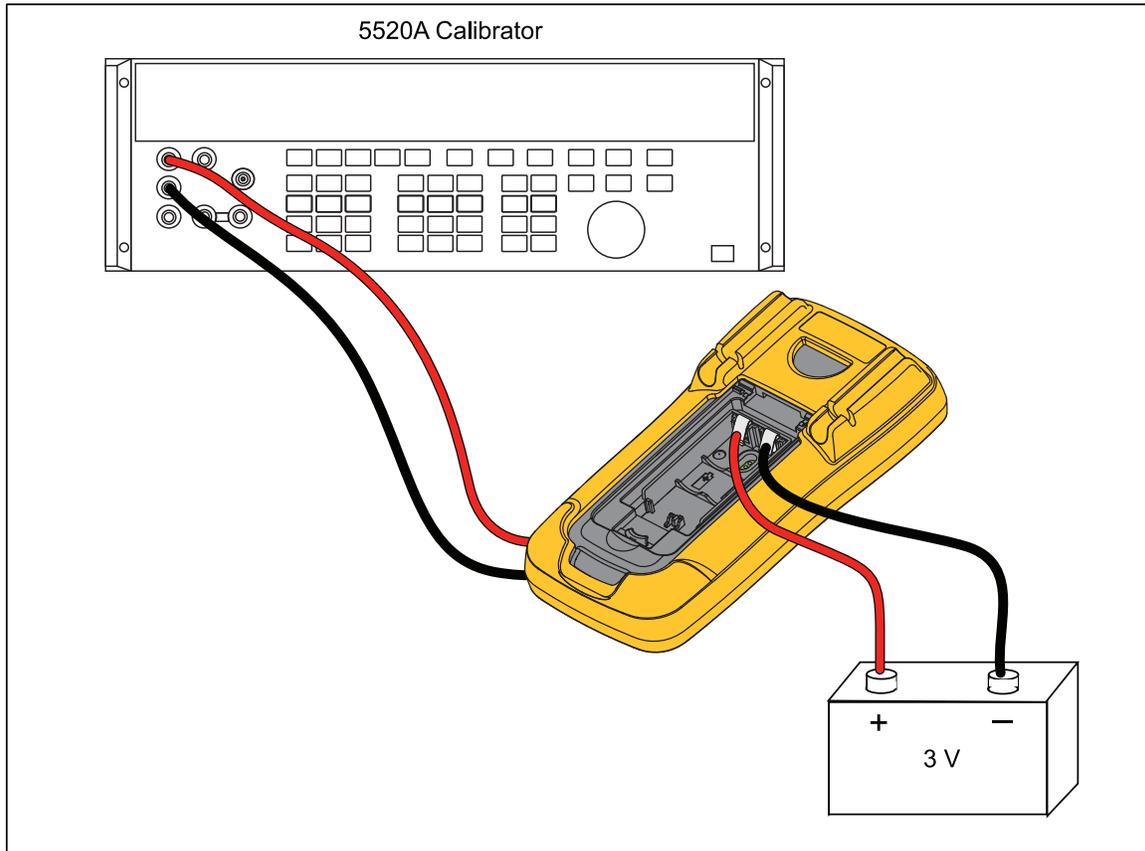
Figure 4. Calibration Connections
